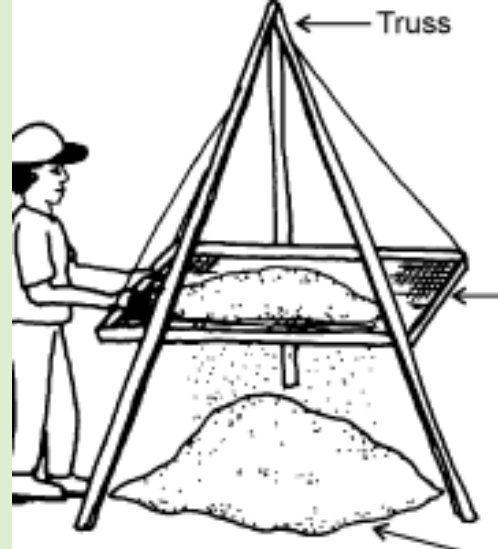
Fig 2 Sieving sand through a hanging frame
