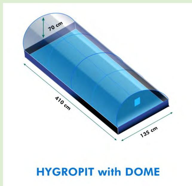
Fig 11 Hygro-pit , lined with plastic, filled with course sand and covered with a plastic dome
