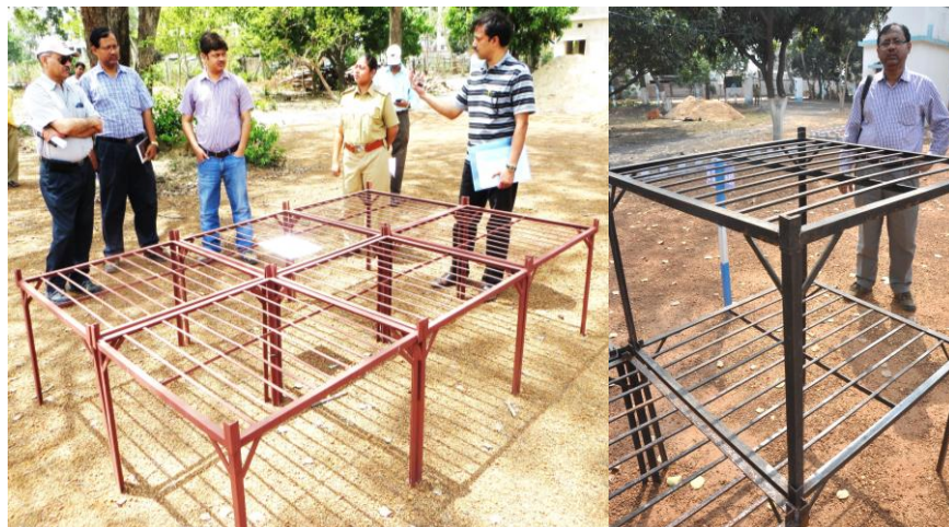
Raised bed elements 85x 85 x 60 cm and stacked for easy transport.
